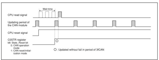
Figure 22.6 With a Wait Time of 3fCAN Before CPU Read
